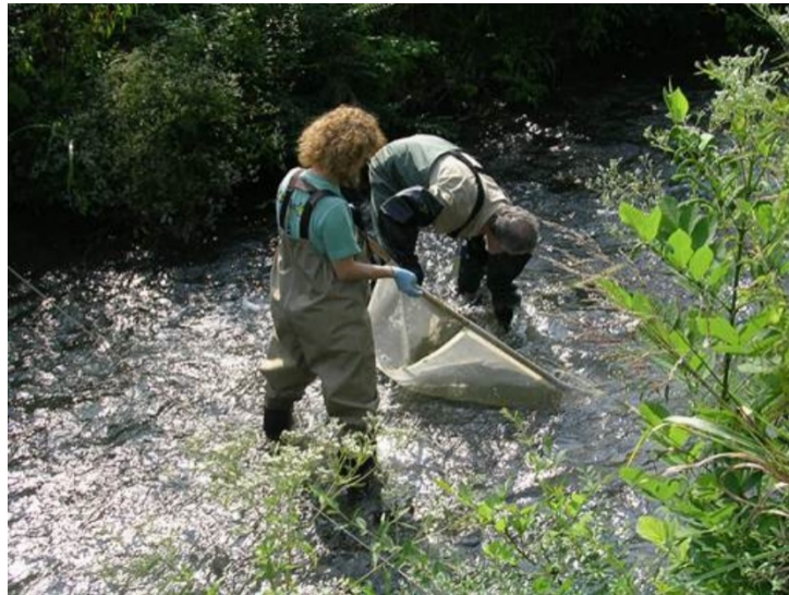
Figure 3.53. Sampling for benthic macroinvertebrates with TDEC protocols
